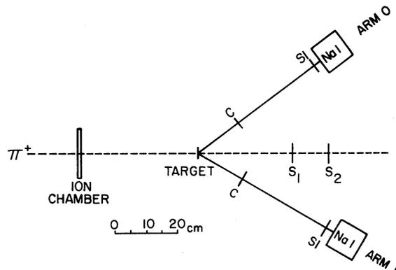
FIG. 1. Experimental apparatus. An ion chamber and two in-beam plastic scintillators monitored the pion beam. Two counter telescope systems measured the scattered pion flux.
