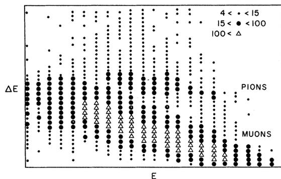
FIG. 2.  $E$  vs  $\Delta E$  spectrum for scattered particles at  $\theta_{\text{lab}} = 30^\circ$ , clearly showing separation between pions and muons.
