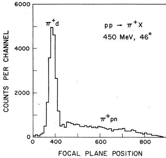
FIG. 1. Pion energy spectrum from the  $\bar{p}p \rightarrow \pi^+d$  reaction. Events from the  $pp \rightarrow pn\pi^+$  reaction are present on the low-energy side of the peak. The background from the carbon in the target has been subtracted.
