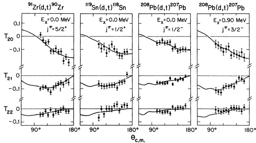
FIG. 4. Measurements of the tensor analyzing powers for sub-Coulomb  $(d, t)$  reactions on  $^{91}\text{Zr}$ ,  $^{119}\text{Sn}$ , and  $^{208}\text{Pb}$ . The curves are DWBA calculations corresponding to the  $D_2$  values listed in Table I.
