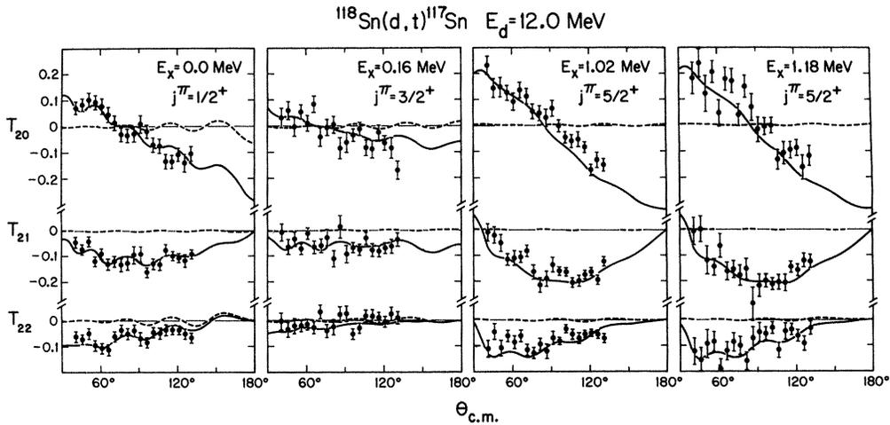
FIG. 7. Measurements of the tensor analyzing powers for  $^{118}\text{Sn}(\vec{d}, t)^{117}\text{Sn}$ . The solid curves are DWBA calculations corresponding to  $D_2 = -0.279$  fm $^2$ , while the dashed curves are calculations which include only the S state.
