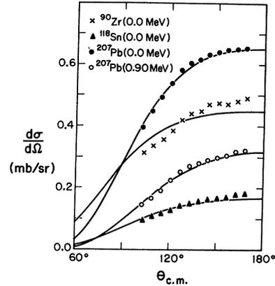
FIG. 3. Cross section measurements for sub-Coulomb ( $d, t$ ) reactions on  $^{91}\text{Zr}$ ,  $^{119}\text{Sn}$ , and  $^{208}\text{Pb}$ . The residual nucleus and the excitation energy are indicated for each angular distribution. The curves are DWBA calculations which have been normalized to obtain the best overall fit to the measurements.
