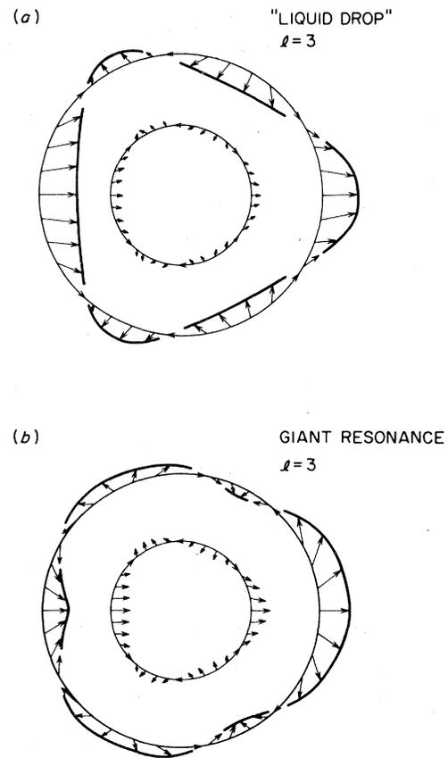
FIG. 8. The displacement vector  $\vec{\mathcal{D}}(\vec{r})$  for the two different types of octupole vibrations. Figure 8(a) is for the liquid-drop vibration and Fig. 8(b) is for the giant octupole resonance at  $\hbar\omega_3 \sim 103 \text{ MeV}/A^{1/3}$ .
