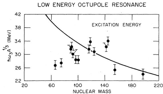
FIG. 5. Comparison of the calculated energies of the liquid-drop octupole state (solid curve) with the experimental data of the isoscalar low-energy octupole resonances. The data points are from the compilation of Ref. 30.
