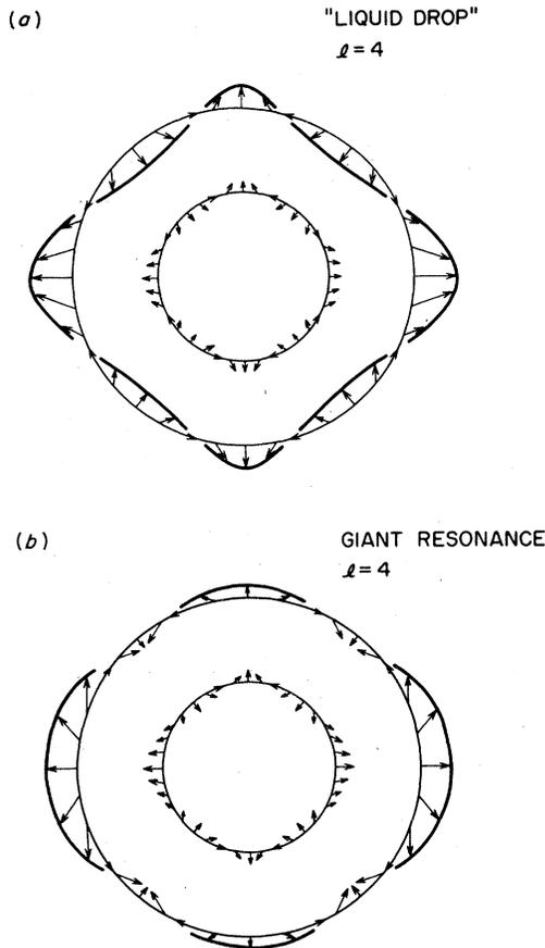
FIG. 9. The displacement vector  $\vec{\xi}(\vec{r})$  for the two different types of hexadecapole vibrations. Figure 9(a) is for the liquid-drop vibration and Fig. 9(b) is for the hexadecapole vibration at  $\hbar\omega_4 \sim 133 \text{ MeV}/A^{1/3}$ .
