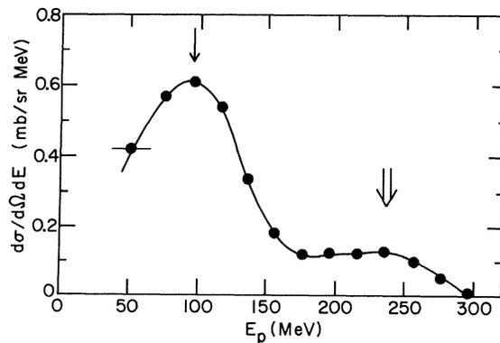
FIG. 3. A typical proton spectrum from  ${}^{12}\text{C}(\pi^+, p)$  at  $30^\circ$ ,  $T_\pi = 220$  MeV. The horizontal bar on the first point indicates the larger bin for these data, the other points are equally spaced. The single arrow shows the energy for proton recoils from  $\pi + N$  scattering, the double arrow for protons from  $\pi + 2N \rightarrow 2N$  absorption.
