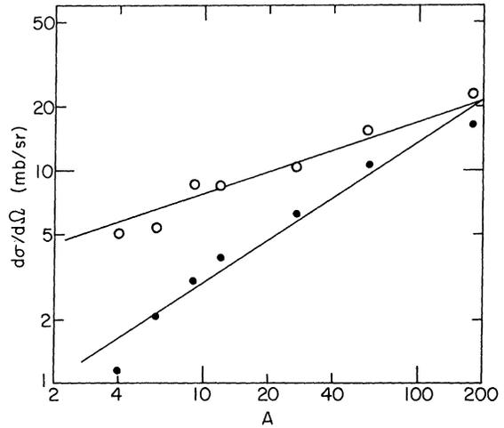
FIG. 6. The  $A$  dependence of high-energy ( $T_p > 160$  MeV) protons from  $\pi^+$  at  $30^\circ$  is shown as open circles. The solid points represent the total angle-integrated proton yield for  $T_p \geq 40$  MeV divided by 100; both curves are for  $T_{\pi^+}=220$  MeV.
