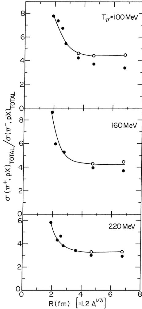
FIG. 11. Ratio of angle integrated total proton yields seen with  $\pi^+$  to those with  $\pi^-$ , as a function of nuclear radius. The open circles include the Coulomb correction  $(T_\pi + V_c)/(T_\pi - V_c)$ , where  $V_c = Ze^2/R$ . The line is to guide the eye.
