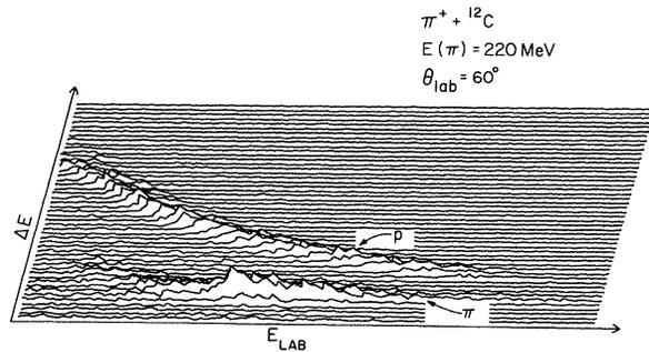
FIG. 2. Three-dimensional display of the  ${}^{12}\text{C} + \pi^+$  data at  $60^\circ$ ,  $T_\pi = 220$  MeV. The ridges of protons and pions are clearly evident; the pions are not stopped in the NaI detector.
