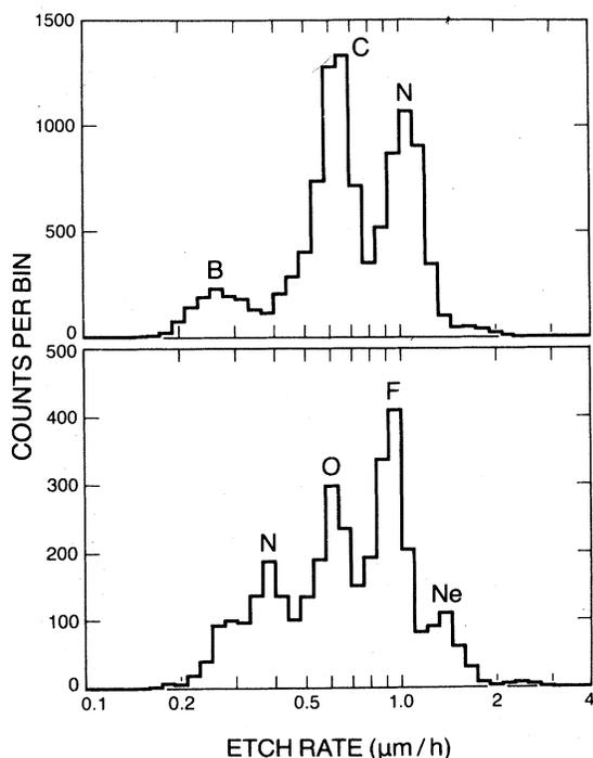
FIG. 1. Charge histograms of elements observed in this experiment. The sensitivity of the plastic detectors was increased by exposure to ultraviolet light. The sensitivity of the detectors used to obtain the top histogram is  $\sim 3$  times higher than the sensitivity of the detectors used to obtain the bottom histogram.
