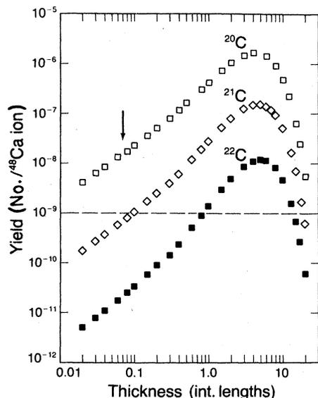
FIG. 4. Calculated yield of neutron-rich carbon ions per  $^{48}\text{Ca}$  ion as a function of target thickness. The calculation assumes a Gaussian mass yield fitted to measured cross sections. The arrow indicates the target thickness for this experiment and that of Ref. 14. The dashed line corresponds to a yield of 10 events with present beam intensities and a detector with collecting power comparable to ours.
