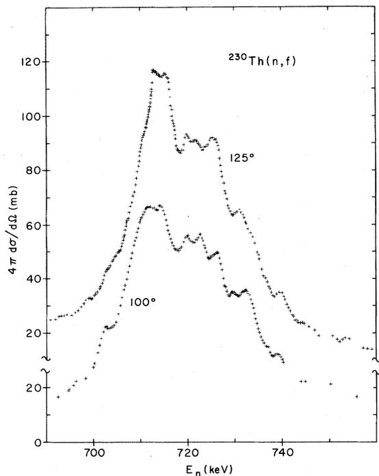
FIG. 2. Experimental results. The points were obtained by digitizing the traces of Fig. 1 and converting them to cross sections relative to the fission cross section of  $^{239}\text{Pu}$ . The uncertainties in the cross section and in the absolute energy calibration are discussed in the text.
