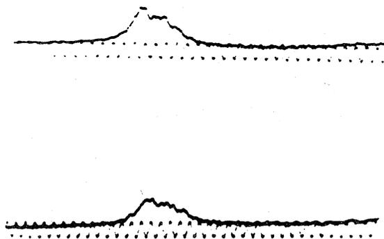
FIG. 1. The oscilloscope traces showing the fission fragment detector responses for 125° (top) and 100° (bottom). Beneath each trace is a 100-MHz sine-wave signal which provides the time calibration and baseline. Time increases from right to left.
