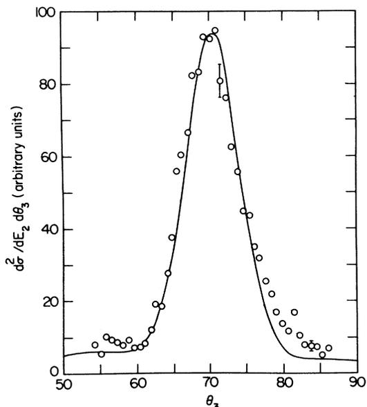
FIG. 2.  ${}^2\text{Li} \Rightarrow 3\alpha$  for  $E_B = 2.0$  MeV. Relative cross section for an  $\alpha$  particle at an angle  $\theta$  that is in time coincidence with an  $\alpha$  particle of energy between 9.9 and 11.4 MeV found at  $90^\circ$  on the opposite side of the target chamber. Experimental uncertainty is indicated by sample error bars. The calculation of the solid curve is described in the text.
