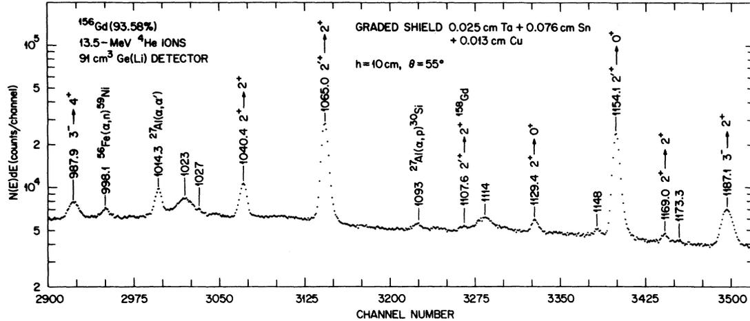
FIG. 1. A section from a 8192-channel pulse-height spectrum of the  $\gamma$  rays from  $^{156}\text{Gd}$  bombarded with 13.5-MeV  $^4\text{He}$  ions.
