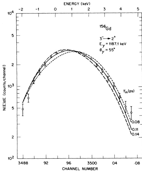
FIG. 2. Detailed comparison of the observed Doppler-broadened shape of the 1187.1-keV  $\gamma$ -ray peak from the  $3^- \rightarrow 2^+$  transition in  $^{156}\text{Gd}$  with calculated shapes for different assumed values of the total mean lifetime of the Coulomb-excited  $3^-$  state.
