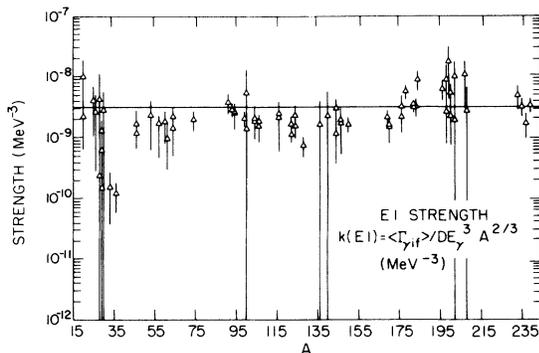
FIG. 1. A plot of the reduced  $E1$  strengths against mass number. The average shown corresponds to 0.043 W.u./MeV.
