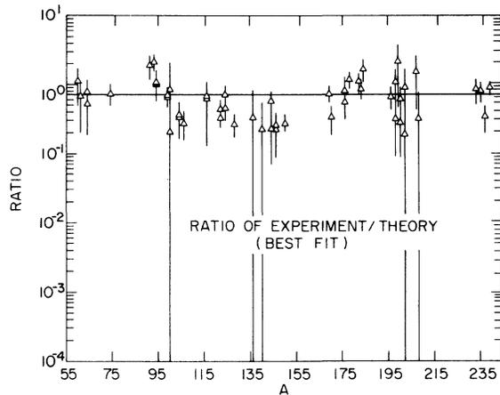
FIG. 3. The ratio of observed  $E1$  strengths, defined as  $\langle \Gamma_{\gamma if} \rangle / D$  to the Lorentz extrapolated values from photoexcitation experiments. An average ratio of 0.7 is shown.
