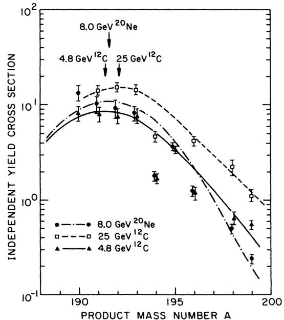
FIG. 1. The isotopic production cross sections for gold products from the reaction of 4.8 and 25.2 GeV  $^{12}\text{C}$  and 8.0 GeV  $^{20}\text{Ne}$  with  $^{209}\text{Bi}$  are shown. The lines represent the best Gaussian fit to each distribution with the arrows showing the distribution centroids.
