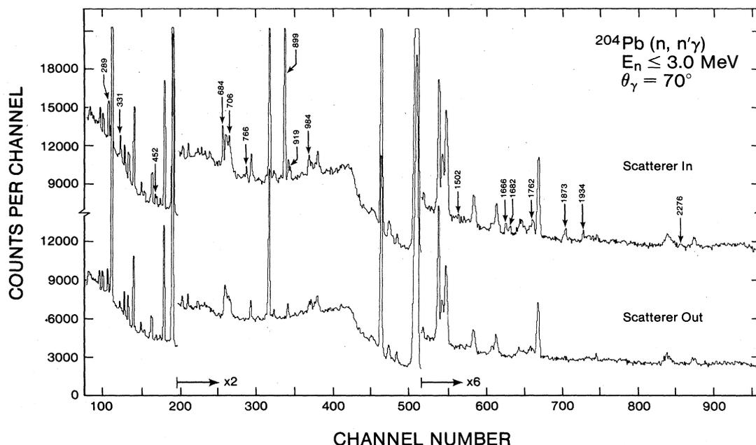
FIG. 1. Sample gamma-ray spectra are shown for scatterer in and scatterer out.  $^{204}\text{Pb}$  gamma-ray energies are given in keV.
