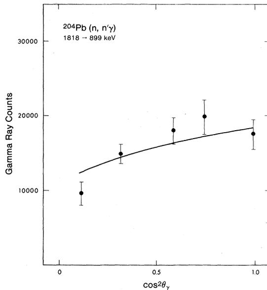
FIG. 3. A sample gamma-ray angular distribution and theoretical fit (Ref. 6) is shown for an initial state spin of 4; the final state is known (Ref. 4) to be  $2^+$ .
