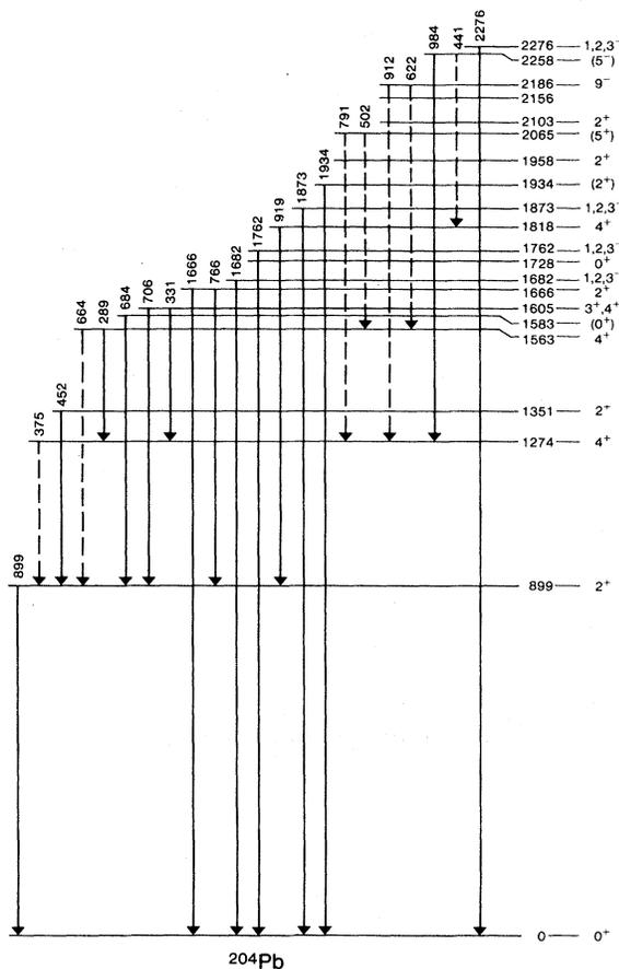
FIG. 2. The level and decay scheme of  $^{204}\text{Pb}$  is shown. The energies are given keV. The gamma-ray energies are those of Refs. 4 and 9, except for the 2276 keV gamma ray, for which the energy is from the present work. The dashed lines refer to previously reported transitions which were not seen in this work. The level spins are from this and previous work.
