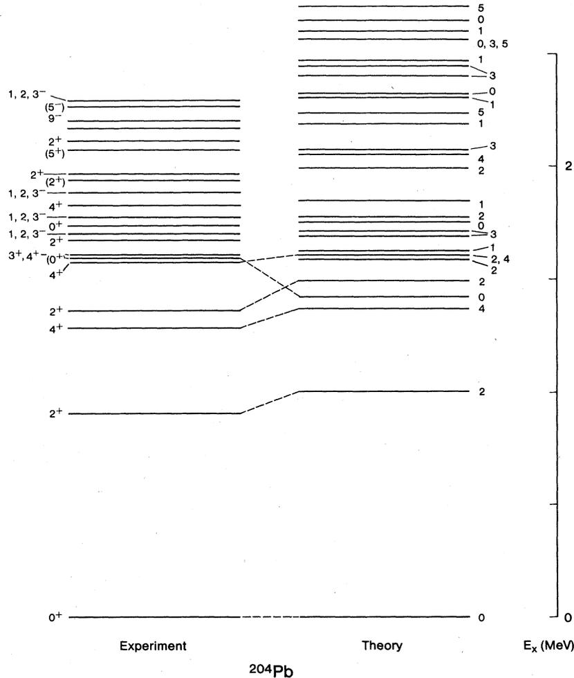
FIG. 5. A comparison of the experimental (Refs. 4,11) and theoretical (Refs. 1, 5)  $^{204}\text{Pb}$  level schemes is shown. Previously unreported levels at 1605 and at 1682, 1762, 1873, and 2276 keV excitation may be the states of  $J^\pi = 1^+$  and  $3^+$  predicted by McGrory (Ref. 5).
