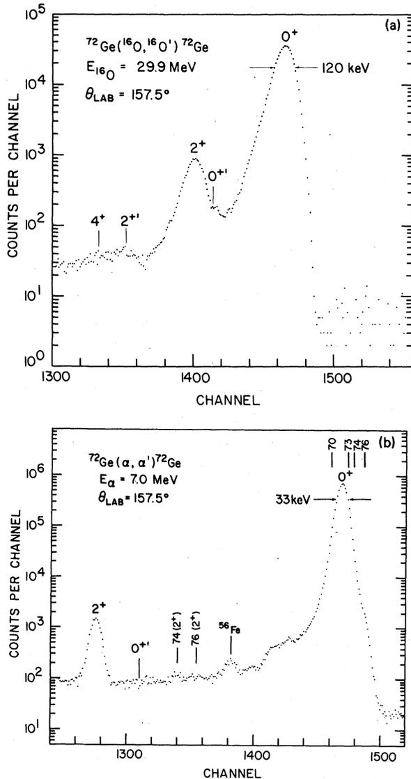
FIG. 1. (a) The  $^{16}\text{O}(29.9 \text{ MeV})$  spectrum from  $^{72}\text{Ge}$  at a scattering angle  $\theta_{\text{lab}} = 157.5^\circ$ . (b) The  $\alpha(7.0 \text{ MeV})$  spectrum of  $^{72}\text{Ge}$  at a scattering angle  $\theta_{\text{lab}} = 157.5^\circ$
