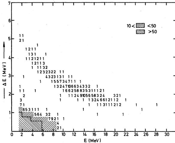
FIG. 1. Two-dimensional  $E$ - $\Delta E$  spectrum of the LRA particles for the photofission of  $^{235}\text{U}$  with 20-MeV bremsstrahlung. In each channel the number of counts is indicated.
