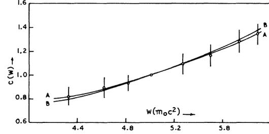
FIG. 7. Experimental shape correction factor  $C(W)$  vs  $W$  for  $\beta_2$  transition as taken from Ref. 5. The theoretical predictions for the typical NME sets (A and B) given in Table V are shown by the smooth curves.
