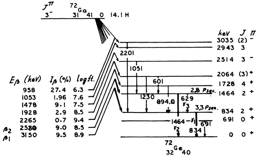
FIG. 1. Partial decay scheme of the ground state decay of  $^{72}\text{Ga}$  as taken from Ref. 1. The  $\beta$ - $\gamma$  cascades of present interest are shown by bold lines.
