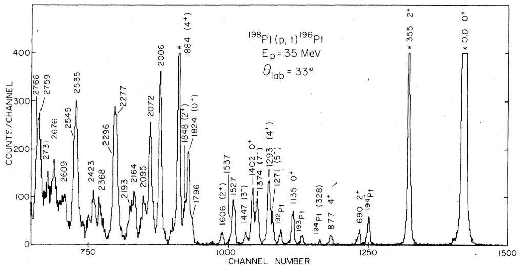
FIG. 1. Triton spectrum at 33° from the <sup>198</sup>Pt(p,t)<sup>196</sup>Pt reaction. Data obtained with a position sensitive delay-line counter (FWHM  $\approx 15$  keV) in the focal plane of the MSU Enge split-pole spectrograph. "\*" above peak indicates peak height has been cut off at maximum value shown on vertical scale.
