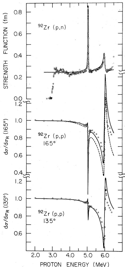
FIG. 1.  $^{92}\text{Zr}(p,n)$  strength function and  $^{92}\text{Zr}(p,p)$  differential elastic cross sections normalized to Rutherford. The solid curve is the result of the coupled-channels calculation described in the text. The dashed curve is the result of a coupled-channels calculation performed with real diffuseness of 0.73 fm.
