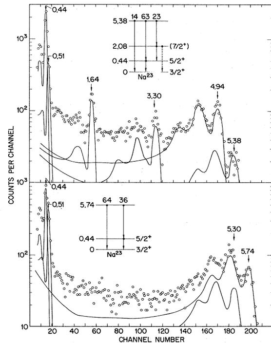
FIG. 8.  $\gamma$ -ray spectra obtained in coincidence with  $\alpha$  particles populating the 5.38- and 5.74-MeV levels of  $\text{Na}^{23}$ .
