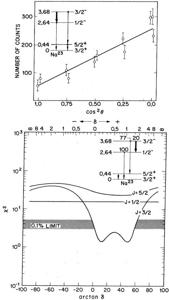
FIG. 5. Summary of the angular distribution obtained for the 1.04-MeV  $\gamma$  ray corresponding to the 3.68  $\rightarrow$  2.64 transition.  $J = \frac{1}{2}$  is ruled out by the known upper limit on the mean life of the level. The upper part of the figure shows the angular distribution as observed with the use of the third NaI(Tl) detector (see text) while the lower part displays the results of the least-squares analysis:  $J = \frac{3}{2}$  is the only spin value allowed by this analysis.
