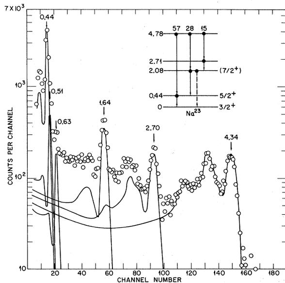
FIG. 7.  $\gamma$ -ray spectra obtained in coincidence with  $\alpha$  particles populating the 4.78-MeV level of  $\text{Na}^{23}$ .
