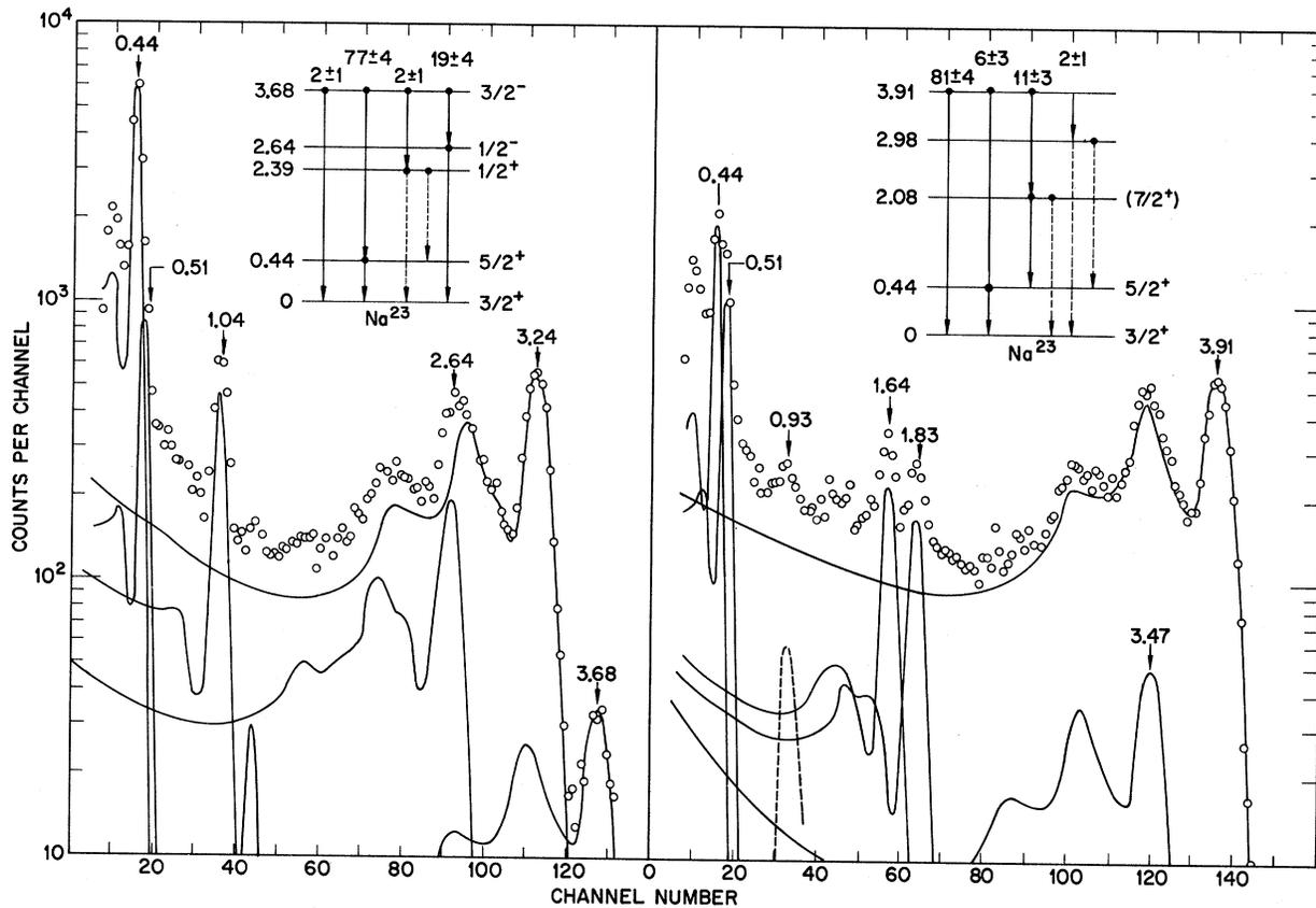
FIG. 4.  $\gamma$ -ray spectra obtained in coincidence with  $\alpha$  particles populating the 3.68- and 3.91-MeV levels of  $\text{Na}^{23}$ . The continuous curves represent the decomposition of each spectrum into its constituent  $\gamma$  rays.
