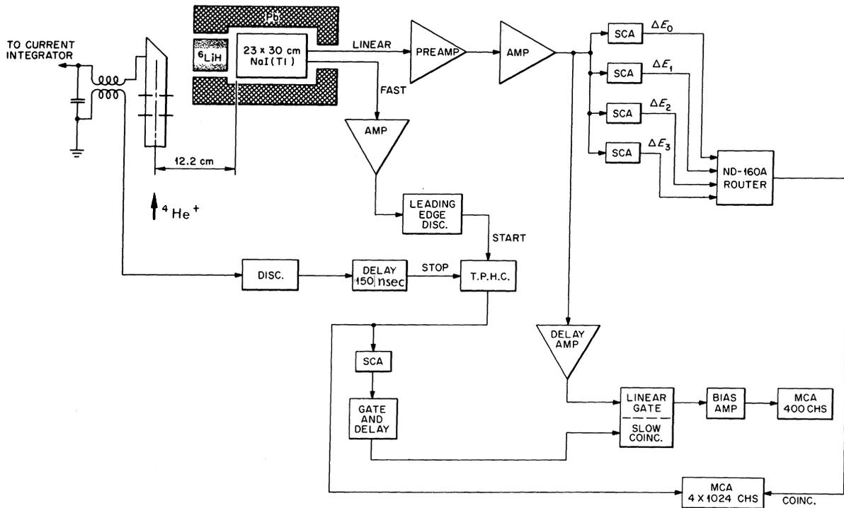
FIG. 1. Electronic circuit used for the  $^{12}\text{C}(\alpha, \gamma)^{16}\text{O}$  capture cross-section measurement. The leading-edge discriminator could be set to trigger at a point equivalent to 2.5 MeV on the pulse; thus, the fast-neutron-induced events could be further separated from the prompt- $\gamma$ -induced events.
