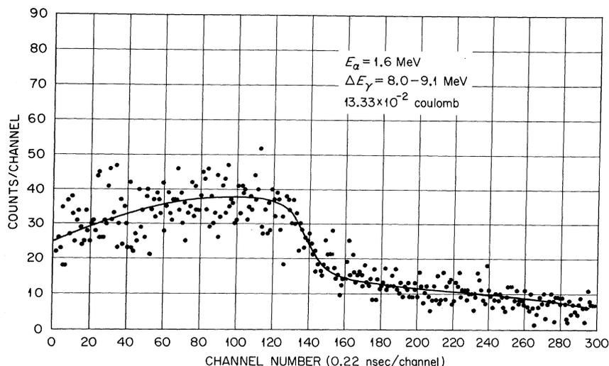
FIG. 8. Time-of-flight pulse-height spectrum at  $E_\alpha = 1.6$  MeV. Note that in this spectrum there is essentially no evidence of a  $\gamma$ -ray-induced peak resulting from the  $^{12}\text{C}(\alpha, \gamma)^{16}\text{O}$  reaction.
