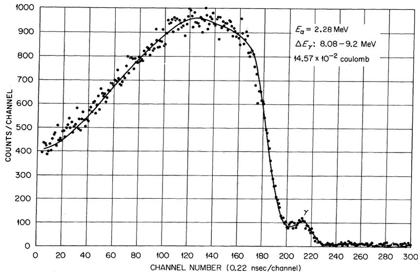
FIG. 6. Pulse-height spectrum for time-of-flight data at  $E_{\alpha} = 2.28 \text{ MeV}$ .
