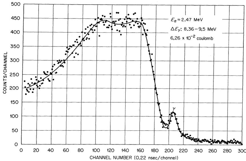
FIG. 5. Pulse-height spectrum for time-of-flight data corresponding to  $\alpha$ -particle energy of 2.47 MeV showing a considerably decreased ratio of  $\gamma$ -ray-induced peak area to fast-neutron-induced peak area as compared to the one observed in Fig. 4.
