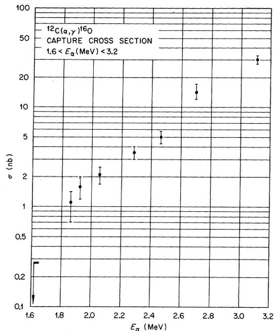
FIG. 9. The  $^{12}\text{C}(\alpha, \gamma)^{16}\text{O}$  capture cross section measured in the present experiment. The errors include the effects due to target-thickness uncertainty, detector-efficiency uncertainty, current integration, statistics, and background subtraction. Refer to text for comparison of data with previous results.
