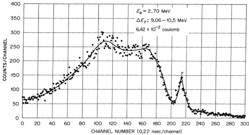
FIG. 4. Time-of-flight pulse-height spectrum at  $E_{\alpha} = 2.70 \text{ MeV}$ . The leading-edge discriminator adjusted to trigger at an energy equivalent to 2.5 MeV. The fast-neutron-induced peak has been broadened toward late-arrival times. Note that the time calibration is 0.22 nsec/channel.
