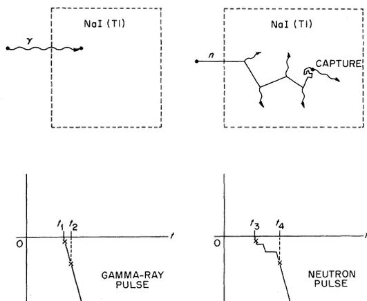
FIG. 2. Schematic representation of 8-10-MeV pulses due to fast neutrons and  $\gamma$  rays in a large NaI(Tl) crystal showing the additional delay of the fast-neutron-induced pulse as a result of inelastic scatterings within the crystal. The time interval  $(t_4 - t_3)$  will be larger than the time interval  $(t_2 - t_1)$ .
