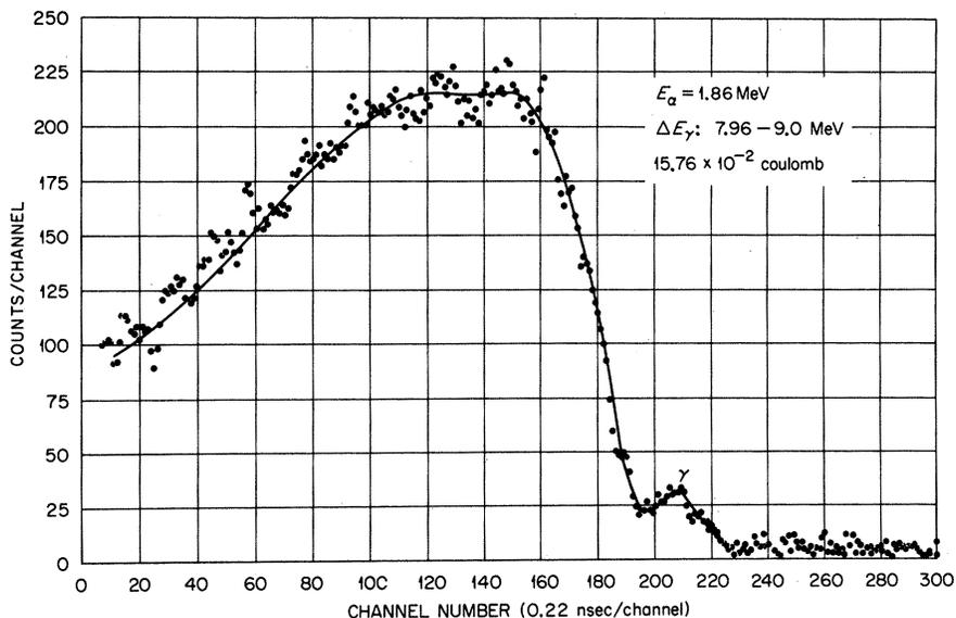
FIG. 7. Time-of-flight pulse-height spectrum at  $E_\alpha = 1.86$  MeV corresponding to an excitation energy in  $^{16}\text{O}$  of 8.6 MeV. The data for this spectrum has been smoothed by averaging in groups of three channels, for all channels containing more than 15 counts.
