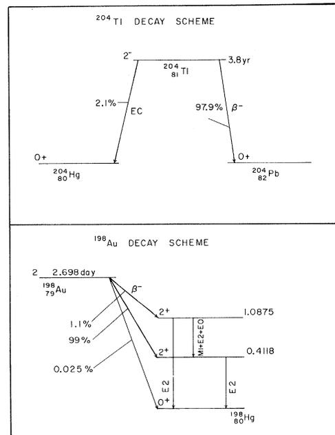
FIG. 1. The decay schemes of <sup>198</sup>Au and <sup>204</sup>Tl.
