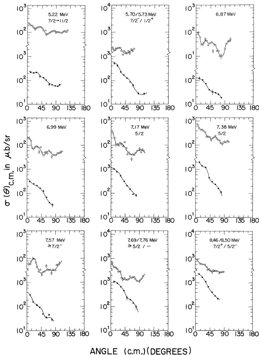
FIG. 3. Particle distributions from the  $^{13}\text{C}(^6\text{Li}, d)$  reaction (open circles) and  $^{13}\text{C}(^7\text{Li}, t)$  reaction (filled circles) leading to states of  $^{17}\text{O}$  between 5- and 8.5-MeV excitation. Representative errors only are shown. The spin-parity assignments are from Table I.
