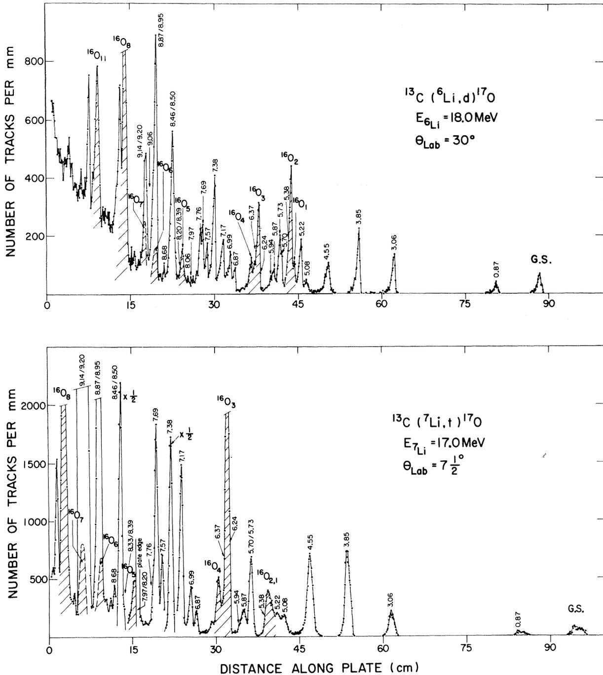
FIG. 1. Deuteron and triton spectra from the  $^{13}\text{C}(^6\text{Li}, d)$  and  $^{13}\text{C}(^7\text{Li}, t)$  reactions. Groups corresponding to states in  $^{17}\text{O}$  are indicated by the corresponding level energies. Those corresponding to states in  $^{16}\text{O}$  are shown cross hatched and arise from  $^{12}\text{C}$  contaminant in the target.
