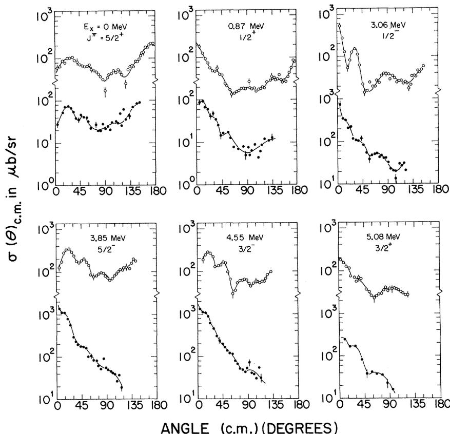
FIG. 2. Particle distributions from the  $^{13}\text{C}(^6\text{Li}, d)$  reaction (open circles) and the  $^{13}\text{C}(^7\text{Li}, t)$  reaction (filled circles) leading to the first six states of  $^{17}\text{O}$ . For clarity, representative errors only are shown. The spin-parity assignments are from Table I.
