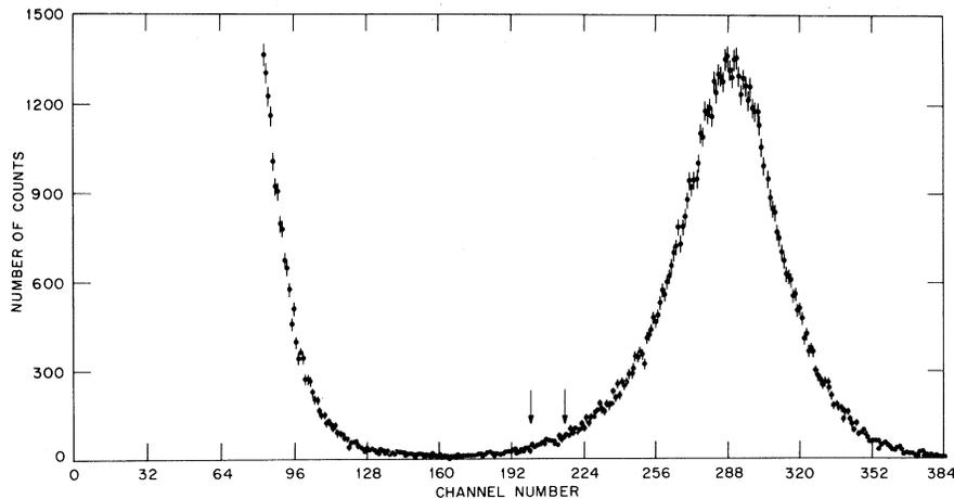
FIG. 2. A typical  $\alpha$ -particle spectrum. The large peak, containing 79 023 counts, is due to the 9.6-MeV state. Vertical arrows indicate the expected positions of peaks due to the 8.87-MeV state.
