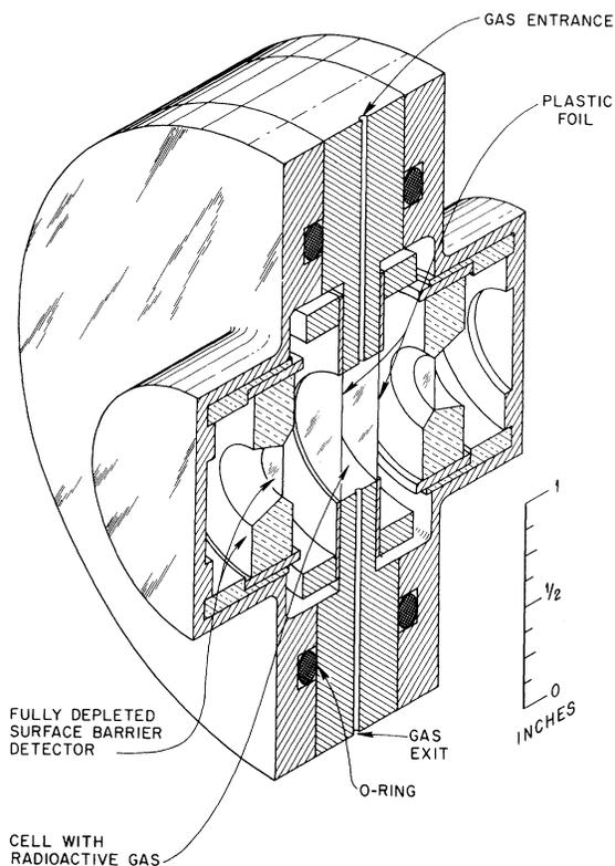
FIG. 1. A simplified view of the counting cell. Bolts, bolt holes, detector electrical connections, interconnecting passages, and other details are not shown.
