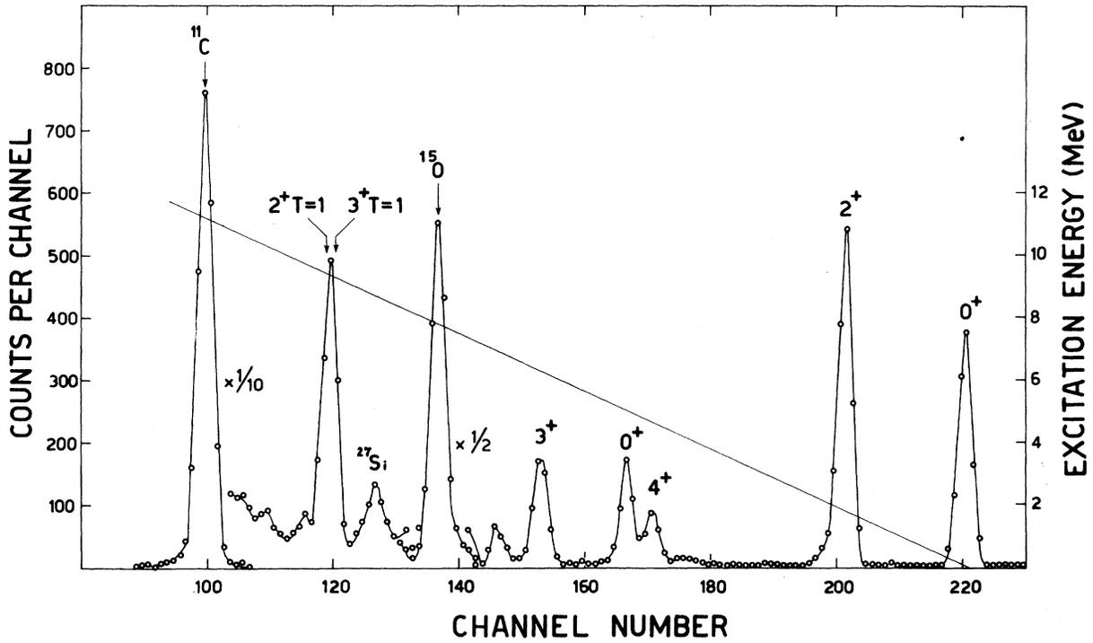
FIG. 2. Deuteron spectrum from the  $^{29}\text{Si}(p, d)^{28}\text{Si}$  reaction at  $\theta_{\text{lab}} = 50^\circ$ . The straight line gives the excitation energy of the residual  $^{28}\text{Si}$  nucleus.
