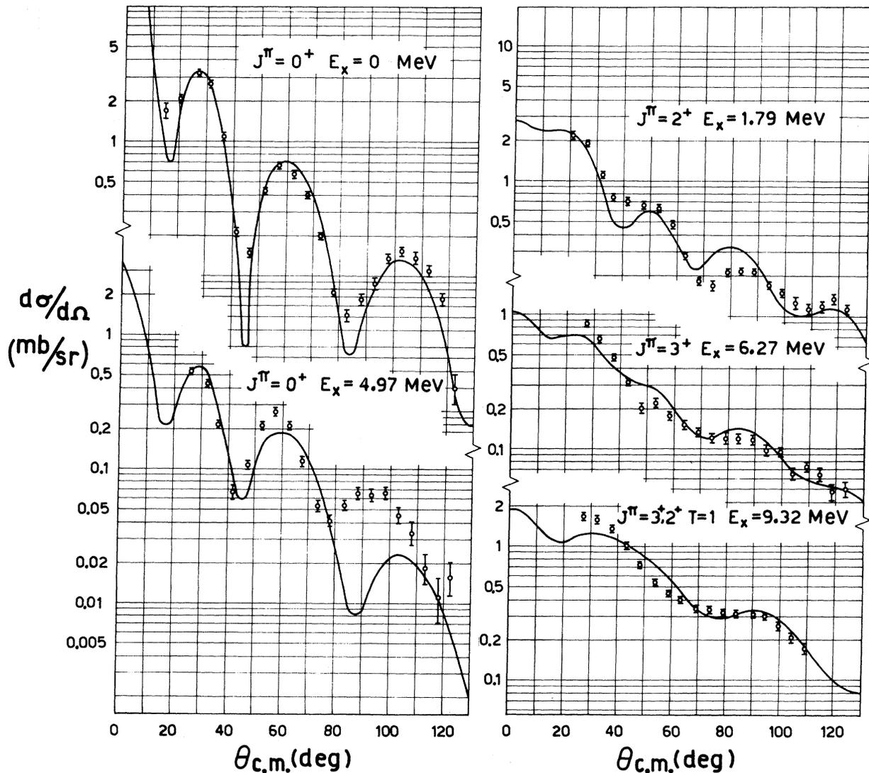
FIG. 4. Theoretical fits to the deuteron angular distributions for the  $^{29}\text{Si}(p,d)^{28}\text{Si}$  reaction using the distorted-wave calculations described in the text. The errors shown are due only to statistical uncertainties.
