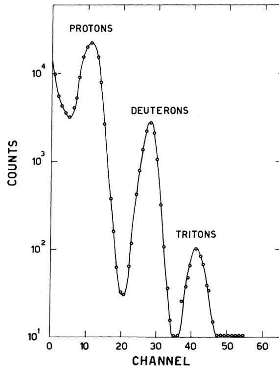
FIG. 1. Mass-identifier-output spectrum for the  $Z=1$  reaction products.
