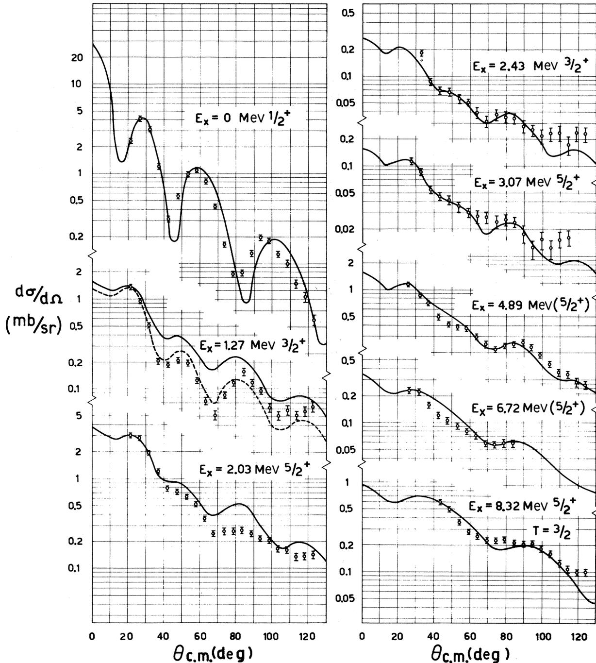
FIG. 5. Angular distributions and distorted-wave curves for the  $^{30}\text{Si}(p, d)^{29}\text{Si}$  reaction. The dashed curve for the transition to the 1.27-MeV state has been obtained using a different binding energy for the transferred neutron ( $-9.35$  MeV). The corresponding spectroscopic factor is 0.44.
