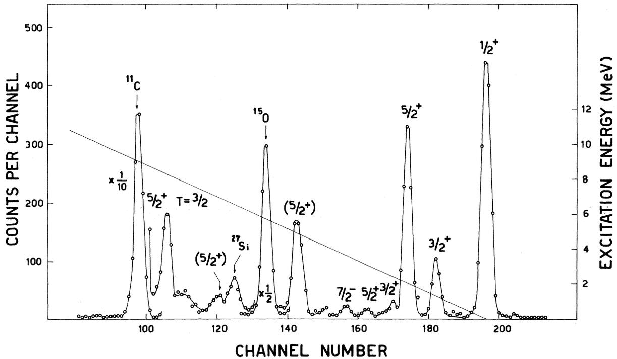
FIG. 3. Deuteron spectrum from the  $^{30}\text{Si}(p, d)^{29}\text{Si}$  reaction at  $\theta_{\text{lab}} = 50^\circ$ . The straight line gives the excitation energy of the residual  $^{29}\text{Si}$  nucleus.
