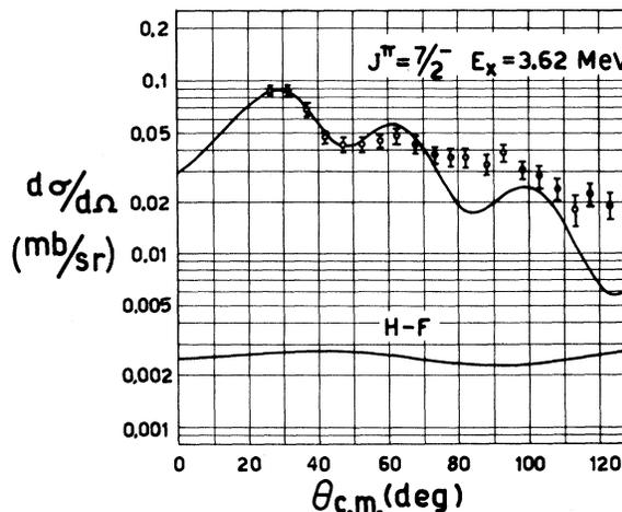
FIG. 7. Differential cross section for the excitation of the 3.62-MeV ( $J^\pi = \frac{7}{2}^-$ ) state of  $^{29}\text{Si}$ . The compound-nucleus contribution is given by the line labeled H-F. The other line is the distorted-wave prediction for  $l_n = 3$ .
