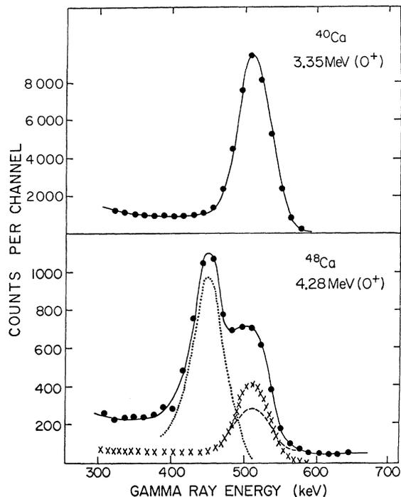
FIG. 1. Gamma-ray spectra in coincidence with protons inelastically scattered from  $0^+$  states of  $^{40}\text{Ca}$  and  $^{48}\text{Ca}$ . The dashed line is the contribution to the 0.511-MeV peak from external pair production of the 3.832-MeV cascade  $\gamma$  ray. The dotted curve shows the 0.452-MeV  $\gamma$  ray; the crossed curve represents the contribution to the 0.511-MeV peak from the internal pair decay of the  $0^+$  state.
