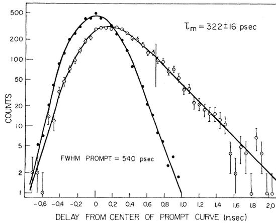
FIG. 2. Prompt and delayed time spectra as gated by protons exciting the 3.832-MeV ( $2^+$ ) and 4.284-MeV ( $0^+$ ) states, respectively.
