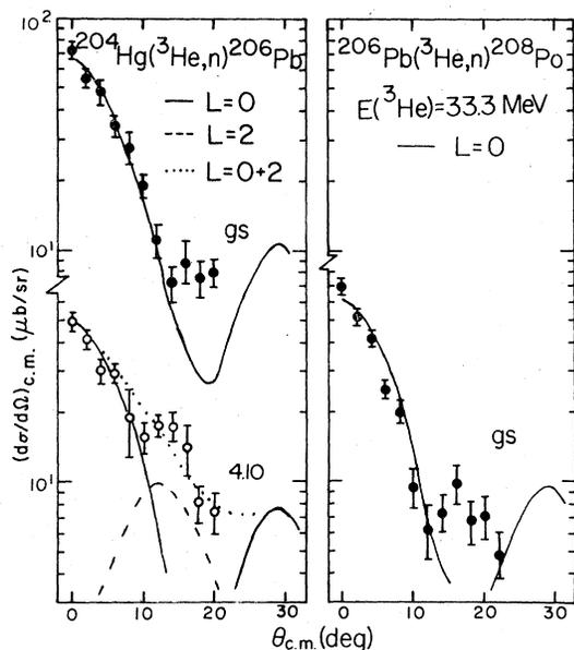
FIG. 2. Angular distributions obtained from the  $^{204}\text{Hg}(^3\text{He},n)^{206}\text{Pb}$  and  $^{206}\text{Pb}(^3\text{He},n)^{208}\text{Po}$  reactions. The solid curves are the results of DWBA calculations described in the text.
