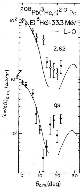
FIG. 3. Angular distributions obtained from the  $^{208}\text{Pb}(^3\text{He},n)^{210}\text{Po}$  reaction. The solid curves are the results of DWBA calculations described in the text.
