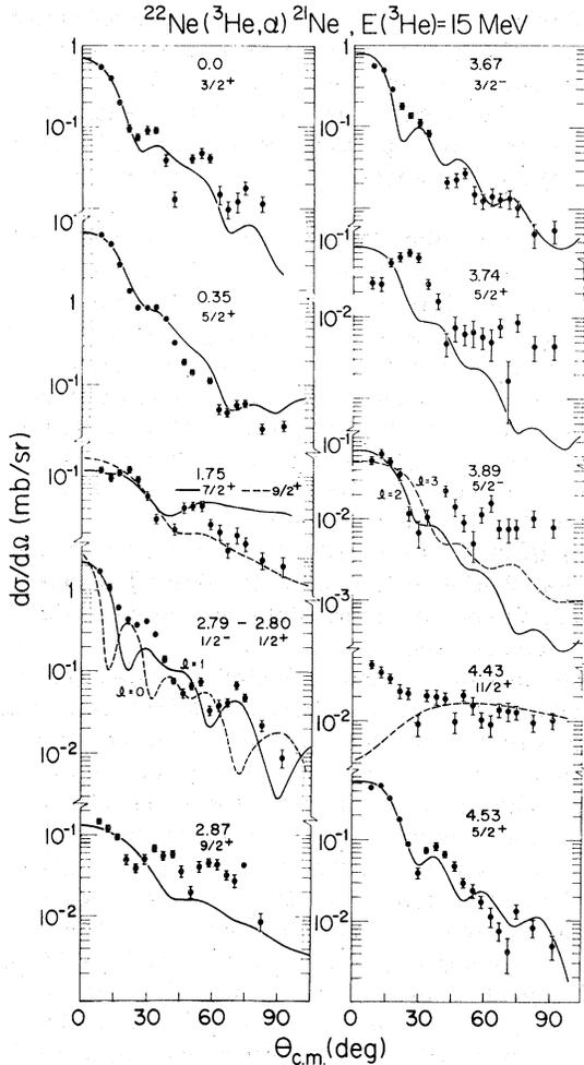
FIG. 2. Angular distributions for the  $^{22}\text{Ne}(^3\text{He}, \alpha)^{21}\text{Ne}$  reaction leading to levels between 0 and 4.6 MeV excitation in  $^{21}\text{Ne}$ . Curves are the results of DWBA calculations.
