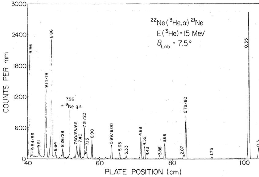
FIG. 1. Spectrum of the  $^{22}\text{Ne}({}^3\text{He}, \alpha){}^{21}\text{Ne}$  reaction at a bombarding energy of 15.0 MeV and a laboratory angle of  $7.5^\circ$ .
