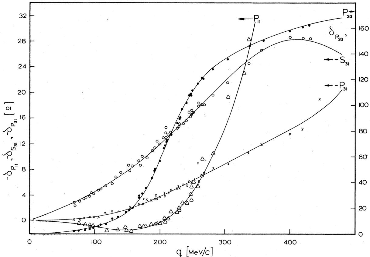
FIG. 1. Phase shifts in degrees for  $S_{31}$ ,  $P_{11}$ ,  $P_{31}$ , and  $P_{33}$  waves. The points have been taken from Refs. 11–17. The full lines are the results of the fits using Eq. (1).
