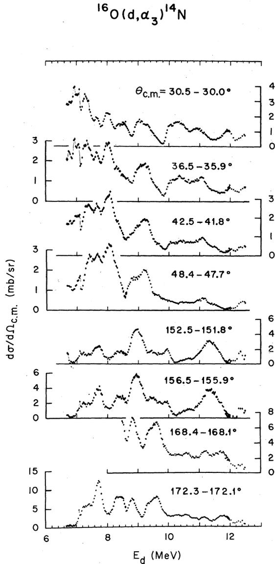
FIG. 1. Differential cross sections for the eight out of 17 laboratory angles ( $\theta_{lab} = 25^\circ, 30^\circ, 35^\circ, 40^\circ, 145^\circ, 150^\circ, 165^\circ, 170^\circ$ ) which showed the largest cross sections. The abscissa is the deuteron energy at the center of the scattering chamber. Center-of-mass angles correspond to the lowest and highest  $E_d$  at  $\theta_{lab}$ . When not shown explicitly, error bars are less than the point size.
