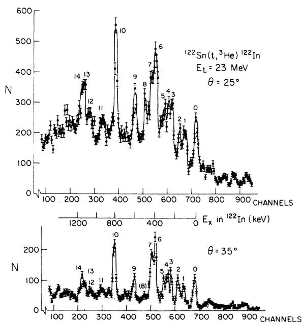
FIG. 1. Spectra of the  $^3\text{He}$  ions from the  $^{122}\text{Sn}(t, ^3\text{He})^{122}\text{In}$  reaction at  $E_t = 23.0$  MeV,  $\theta_{\text{lab}} = 25^\circ$  and  $35^\circ$ ,  $B = 5.4527$  kG. The ordinates show the total number of counts recorded in a five-channel bin. The abscissas show the channel number and the excitation energy in  $^{122}\text{In}$ , in keV. The numbered groups are due to states in  $^{122}\text{In}$ : See Table I.
