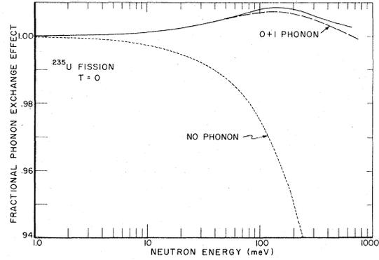
FIG. 1. The quantity  $W'(E) [(E - E_0)^2 + \frac{1}{4}\Gamma^2]$ , which is the ratio of the  $^{235}\text{U}$  fission cross section with phonon exchange to the rigidly bound case, is shown as a function of neutron energy for temperature  $T=0$  K. The dotted line shows the no-phonon-exchange portion. The dashed line shows the cumulative total of zero and one phonon exchange and the solid line the total of all phonon-transfer processes.
