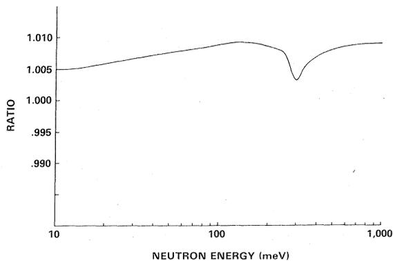
FIG. 5. The fractional phonon exchange effect for the fission cross section of  $^{235}\text{U}$  is shown as calculated for Fig. 4.
