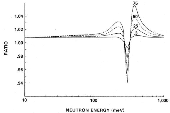
FIG. 2. The fractional phonon exchange effect for the fission cross section of  $^{239}\text{Pu}$  is shown multiplied by the unbroadened Breit-Wigner denominator. For the Einstein model an  $\epsilon = 14$  meV is assumed. The four curves show the effect as a function of temperature in meV. No influence of phonon transfer on  $\Gamma_n$  is included.
