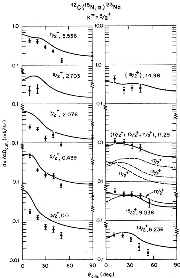
FIG. 2. Energy averaged experimental (36–39.2 MeV) and HF calculated angular distributions for the known and proposed members of the  $K^\pi = \frac{3}{2}^+$  rotational band of  $^{23}\text{Na}$ . The lines indicate the HF predicted  $\sigma(\theta)$  with the solid line indicating that obtained with the preferred spin.
