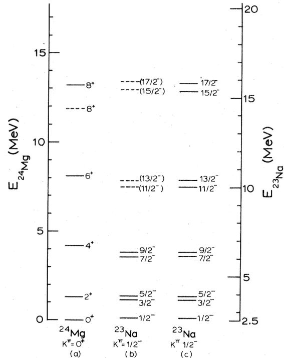
FIG. 8. Comparison of the normalized excitation energies for (a) the ground state members of  $^{24}\text{Mg}$ , (b) known and proposed members of the  $K^\pi = \frac{1}{2}^-$  band of  $^{23}\text{Na}$ , and (c) predicted energies from Eq. (1) in the text with  $\hbar^2/2\mathcal{I} = 179$  keV and  $a' = 0.85$ .
