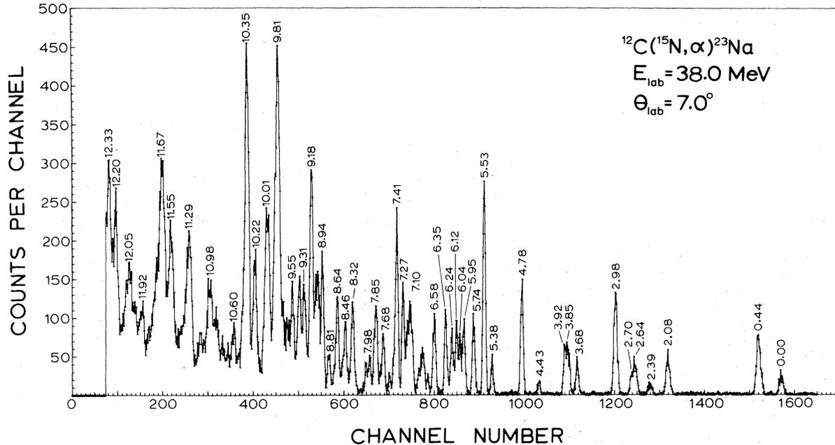
FIG. 1. Typical high resolution spectrum for the  $^{12}\text{C}(^{15}\text{N}, \alpha)^{23}\text{Na}$  reaction. The excitation energies are noted.
