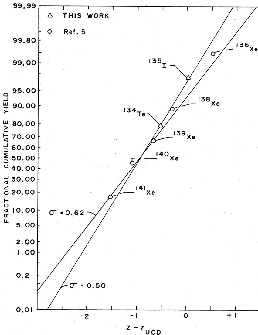
FIG. 4. A plot of  $Z - Z_{UCD}$  as a function of FCY for  $^{252}\text{Cf}$  spontaneous fission.
