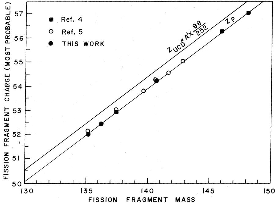
FIG. 3. A plot showing the comparison of  $Z_{UCD}$  and  $Zp$  in the spontaneous fission of  $^{252}\text{Cf}$ .
