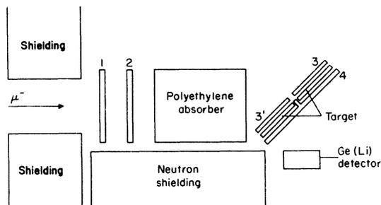
FIG. 1. Block diagram of muon telescope including the position of the Ge(Li) muonic x-ray detector.
