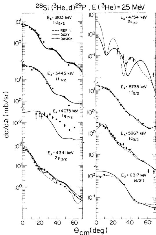
FIG. 1. Angular distributions for the reaction  $^{28}\text{Si}(^3\text{He},d)^{29}\text{P}$  leading to unbound states of  $^{29}\text{P}$ . Data are from Ref. 1. Curves were calculated with the unbound stripping code DOXY (Ref. 5). Resulting spectroscopic factors are listed in Table I.
