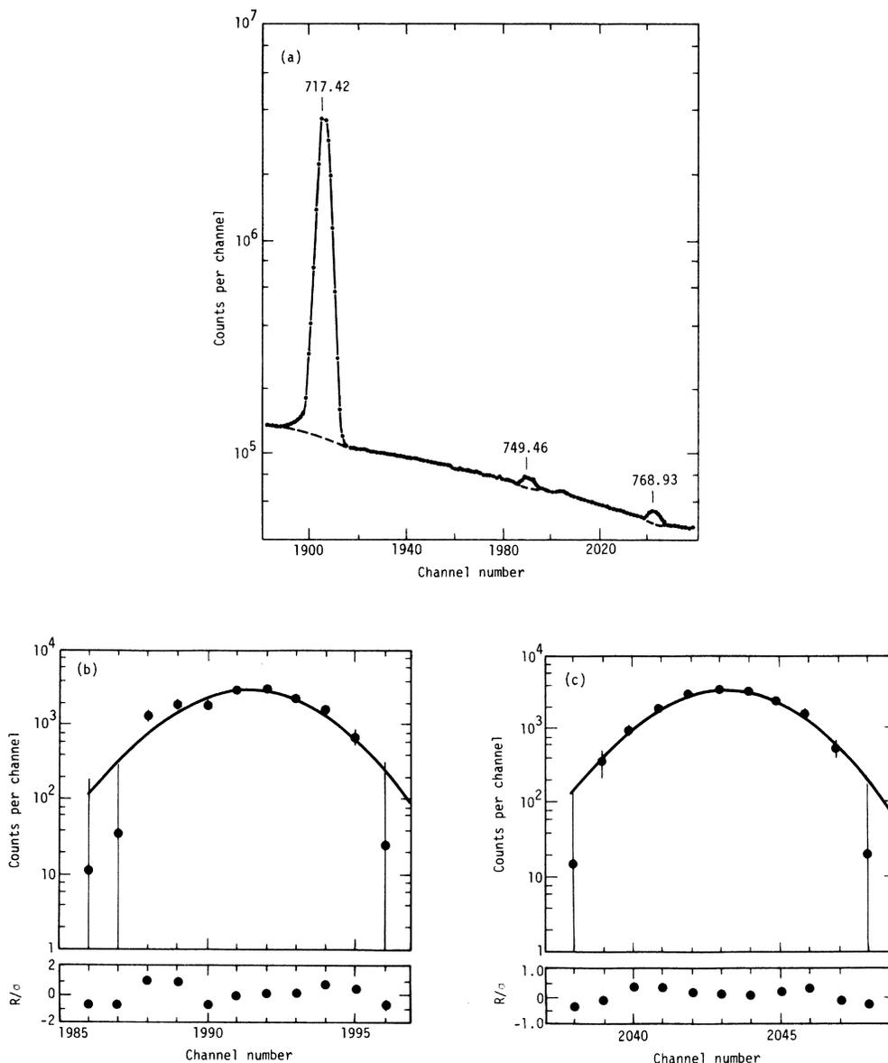
FIG. 1. The  $\gamma$ -ray spectrum of  $^{185}\text{Os}$  decay taken with 10 mm of Pb as an absorber between the source and detector: (a) region from 700 to 800 keV, (b) fit of GAMANAL peak shape (less background) to the 749.46-keV photopeak, and (c) fit of GAMANAL peak shape (less background) to the 768.93-keV photopeak.
