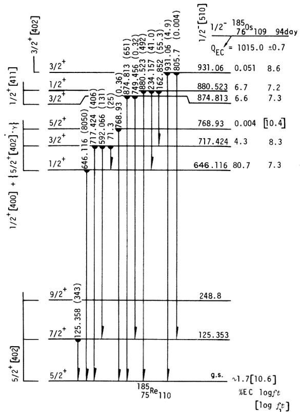
FIG. 3. Decay scheme for  $^{185}\text{Os}$ .
