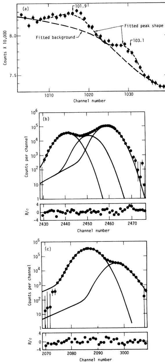
FIG. 2. Selected photopeaks in the spectra of  $^{183}\text{Re}$  decay: (a) region showing the 101.9- and 103.1-keV photopeaks, (b) fit of GAMANAL peak shape to the 244.27-, 245.25-, and 248.06-keV triplet, (c) fit of GAMANAL peak shape to the 208.81- and 209.89-keV doublet. For the fit in (b) and in (c), parameters for peak shape were determined from several single photopeaks within the same spectrum.
