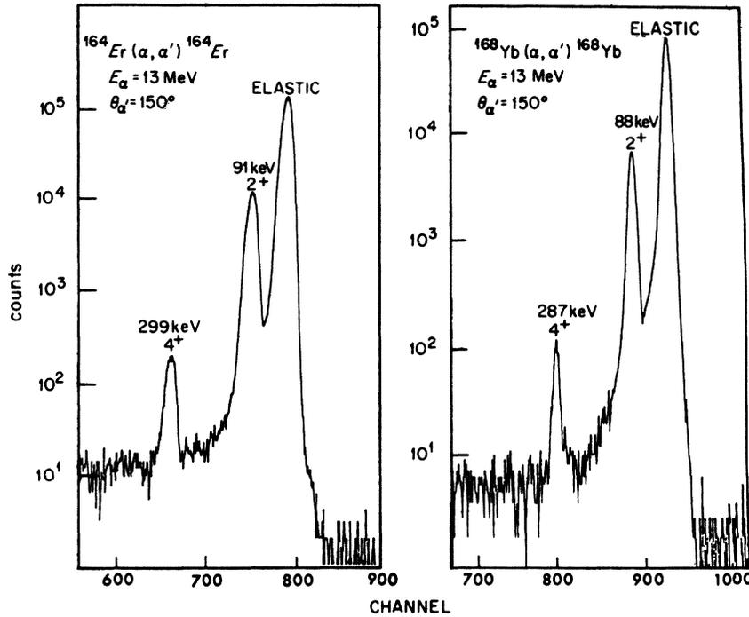
FIG. 1. Spectra of  $\alpha$  particles scattered from  $^{164}\text{Er}$  and  $^{168}\text{Yb}$ .
