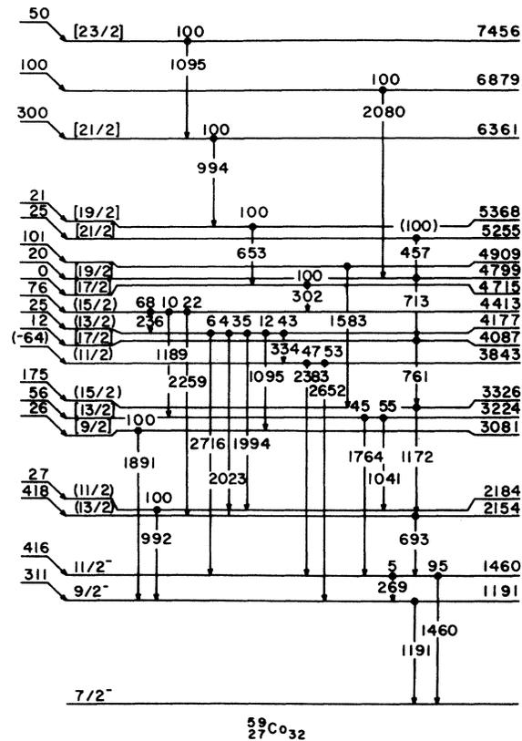
FIG. 8. Level scheme for  $^{59}\text{Co}$  deduced from observation of  $\gamma$  rays from the  $^{48}\text{Ca}(^{15}\text{N}, 4n)^{60}\text{Co}$  reaction. The notation is similar to that of Figs. 1 and 6. Only the yrast (or near-yrast) levels observed in the present studies are shown. Data on the  $\gamma$ -ray transitions are given in Table V.
