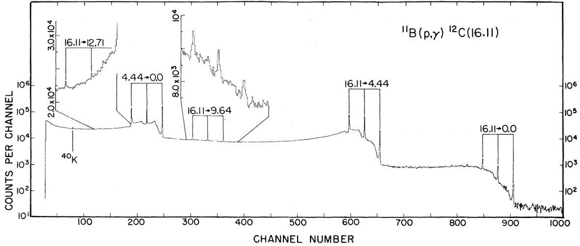
FIG. 6. Spectrum of  $\gamma$  rays from the 163 keV  $^{11}\text{B}(p, \gamma) ^{12}\text{C}(16.11)$  resonance observed in a 15% Ge(Li) detector.
