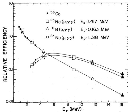
FIG. 7. Measured efficiency of the Ge(Li) detector. The procedure used to obtain these points is described in the text. The  $^{11}\text{B}(p, \gamma)$  points at  $E_\gamma = 16.1$  MeV were only used to obtain the ratios of the single escape and double escape peaks to the full energy peaks.
