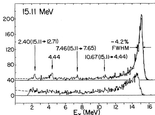
FIG. 5. Spectrum of  $\gamma$  rays in coincidence with protons from the  $^{10}\text{B}(^3\text{He}, p)^{12}\text{C}(15.1)$  reaction. The spectrum of  $\gamma$  rays accepted by the anticoincidence shield is shown above the spectrum rejected by the shield.
