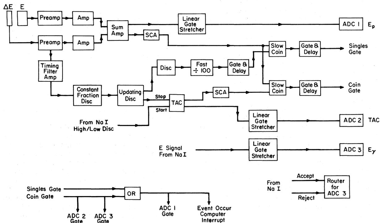
FIG. 1. Block diagram of the electronics used in the  $^{10}\text{B}(^3\text{He}, p\gamma)$  coincidence experiment.
