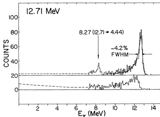
FIG. 3. Spectrum of  $\gamma$  rays in coincidence with protons from the  $^{10}\text{B}(^3\text{He},p)^{12}\text{C}(12.7)$  reaction. The spectrum is not shown below  $E_\gamma \sim 7$  MeV due to strong background  $\gamma$  rays. The spectrum accepted by the anticoincidence shield is shown above the spectrum rejected by the shield.
