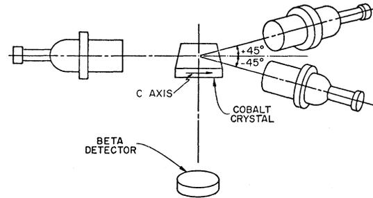
FIG. 3. A schematic representation of the detector geometry showing the three NaI  $\gamma$  detectors in the horizontal plane of crystal at angles of  $-45^\circ$ ,  $+45^\circ$ , and  $180^\circ$  to the  $c$  axis of the cobalt crystal. The  $\beta$  detector is located below the crystal.
