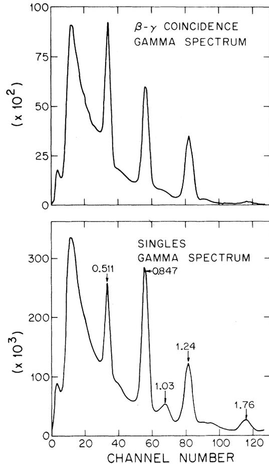
FIG. 5. The  $\gamma$  spectra for  $\beta$ - $\gamma$  coincidences and for  $\gamma$  singles are shown in the two graphs. The 0.511-MeV peak from  $\beta$  annihilation and the 0.847- and 1.24-MeV  $\gamma$  peaks are clearly visible on the coincidence spectrum. The 1.03- and the 1.76-MeV  $\gamma$  peaks from electron capture are also visible in the singles spectra.
