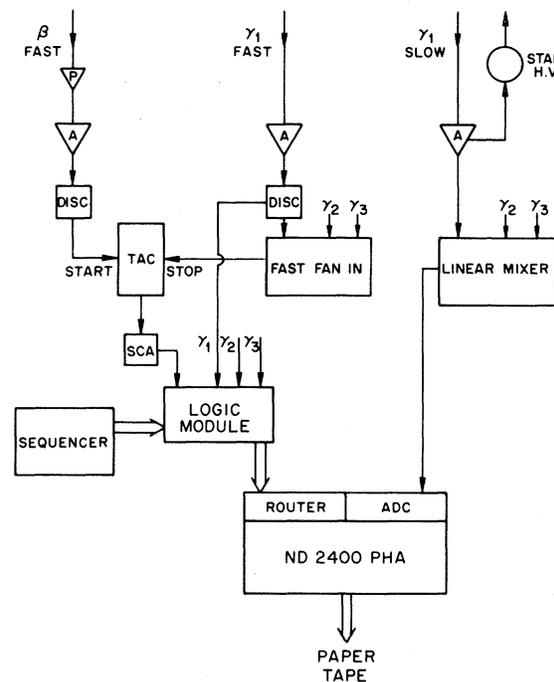
FIG. 4. A block diagram of the counting electronics.
