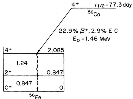
FIG. 1. Partial decay scheme for <sup>56</sup>Co showing the  $\beta$  and the two  $\gamma$  transitions used in our analysis. Not shown are many higher levels which feed these levels by electron capture and subsequent  $\gamma$  emission.
