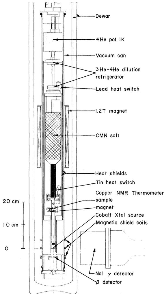
FIG. 2. A schematic representation of the cryogenic apparatus.
