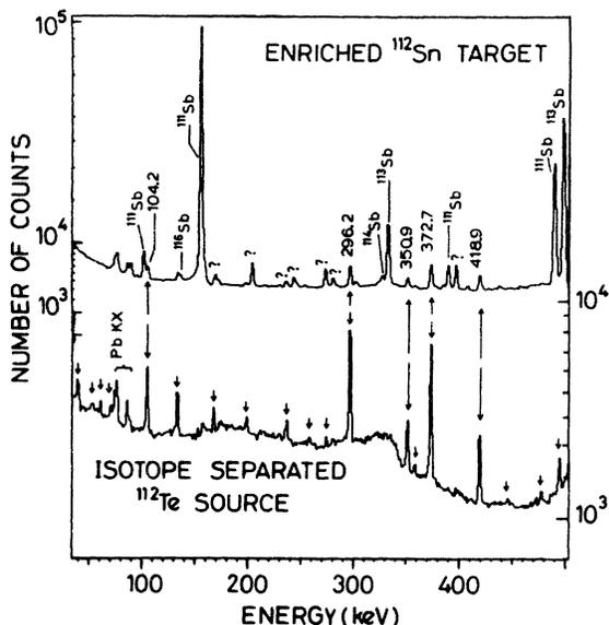
FIG. 1. Part of the  $\gamma$  ray spectrum of  $^{112}\text{Te}$ , measured on sources produced on enriched targets and on isotope separated sources. The  $^{112}\text{Te}$   $\gamma$  rays are denoted by arrows. Only the most intense  $^{112}\text{Te}$   $\gamma$  rays are visible in the upper spectrum.
