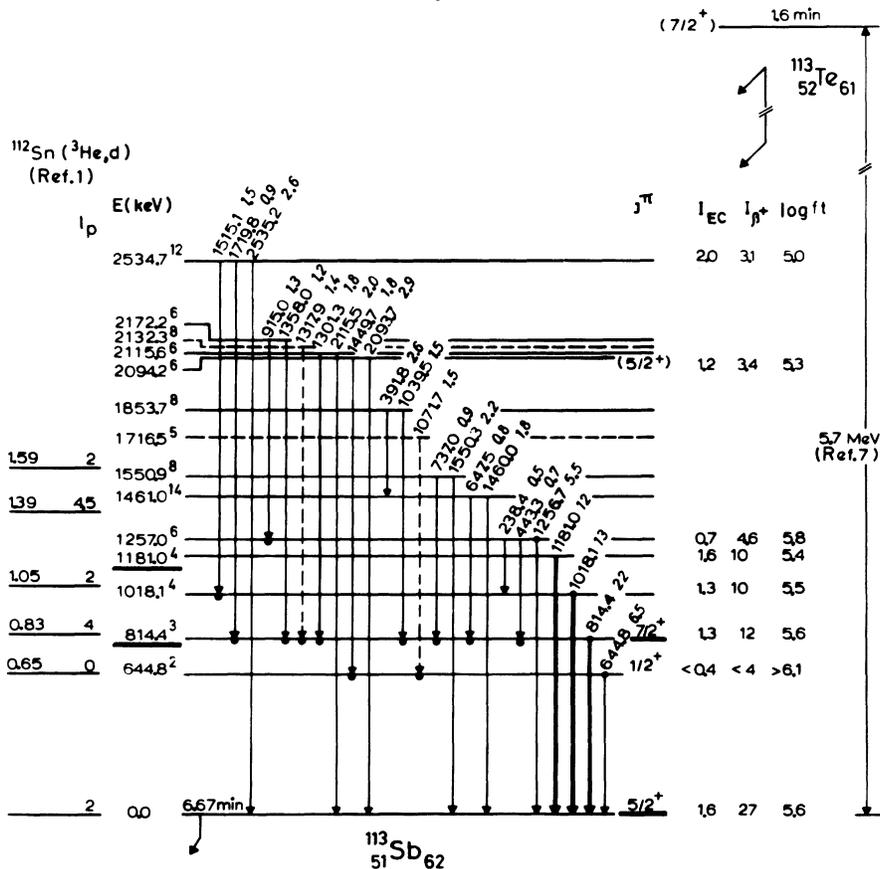
FIG. 6. The decay scheme of  $^{113}\text{Te}$ .
