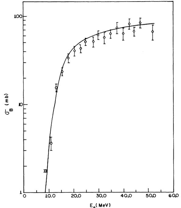
FIG. 2. Bremsstrahlung induced fission yield  $\sigma_B$  of  $^{238}\text{U}$  as function of the maximum photon energy  $E_0$ . The solid line represents the yield curve obtained by folding in the photofission cross section of  $^{238}\text{U}$  (as shown in Fig. 3) with the bremsstrahlung spectrum for a thin radiator (Ref. 17).
