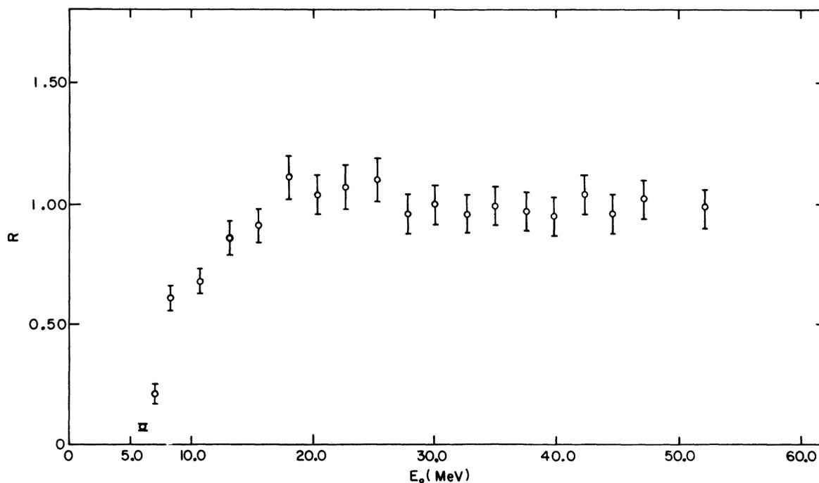
FIG. 5. The relative contribution of the E1 excitation with respect to the total electroexcitation process, as defined in Eq. (6) of the text by the ratio  $R$ , is plotted as a function of the incident electron energy  $E_0$ .
