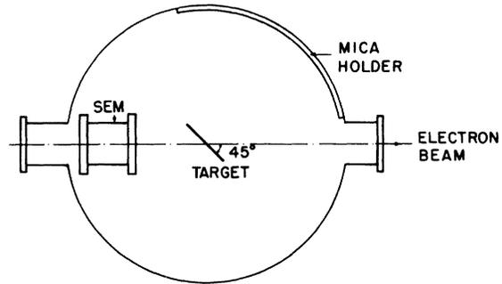
FIG. 1. A simple illustration of the target geometry used in the experiment.
