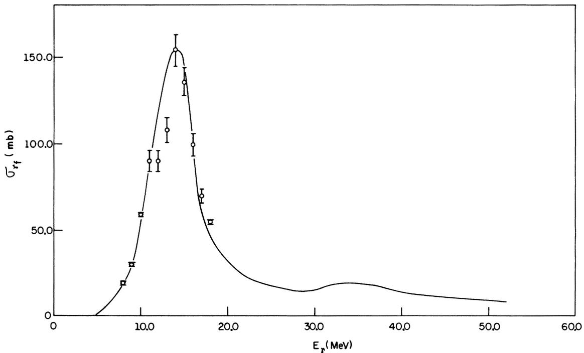
FIG. 3. Photofission cross section  $\sigma_{\gamma f}$  of  $^{238}\text{U}$  as a function of photon energy  $E_\gamma$  is shown by the solid curve obtained by the unfolding of the bremsstrahlung induced fission yields as described in the text. The experimental points shown are the monochromatic photon cross sections of Veyssière *et al.* (Ref. 29).
