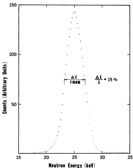
FIG. 1. Energy distribution of the 25-keV neutron filtered beam at the NBS 10-MW reactor.
