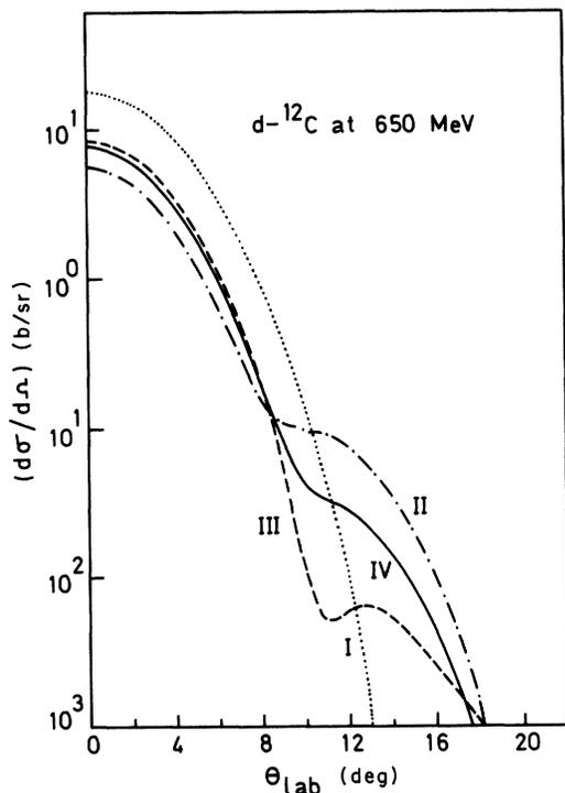
FIG. 1.  $d-^{12}\text{C}$  elastic differential cross section at 650 MeV as a function of the laboratory scattering angle. The curves I, II, III, and IV are the results of retaining terms up to the first, second, third, and fourth order scattering, respectively, in the Glauber expansion.
