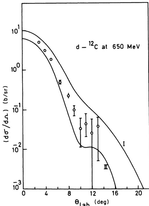
FIG. 3. Curve I is the differential cross section resulting from the choice of the maximum experimentally allowed values of  $\sigma$  and  $\alpha$  and the minimum value of  $\beta^2$ , i.e.,  $\sigma=30.9$  mb,  $\alpha=0.525$ ,  $\beta^2=2.7$   $(\text{GeV}/c)^{-2}$ . The complementary set of values, i.e.,  $\sigma=25.9$  mb,  $\alpha=0.325$ , and  $\beta^2=3.3$   $(\text{GeV}/c)^{-2}$ , leads to curve II.
