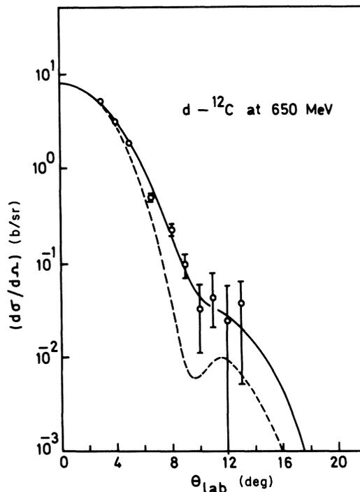
FIG. 2. The solid curve represents our results obtained by including terms up to the fourth order in the Glauber series; the dashed curve is the result of using a  $p-^{12}\text{C}$  optical potential and the experimental points are from Ref. 6.
