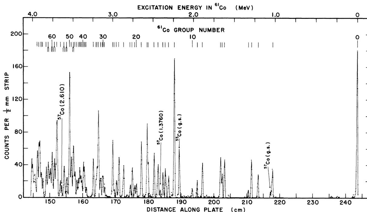
FIG. 3. A typical spectrum from the  $^{64}\text{Ni}(p, \alpha)^{61}\text{Co}$  reaction. The bombarding energy was 14 MeV and the observation angle  $140^\circ$ . Group numbers correspond to those in Table III. Contaminant groups are labeled with the symbol and excitation energy of the residual nucleus. The analysis was terminated at group 69.
