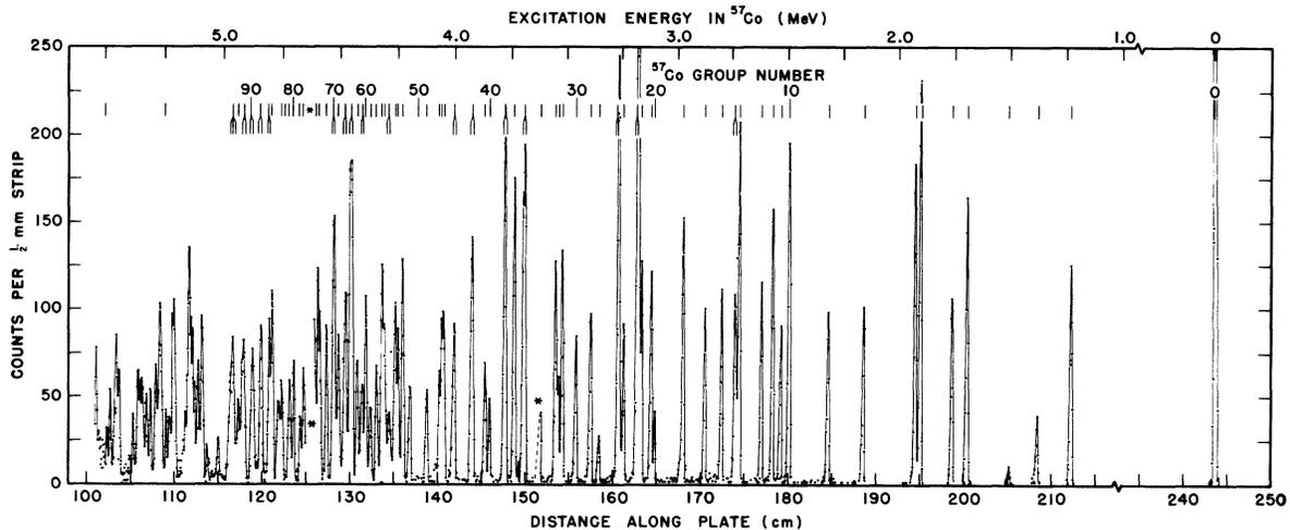
FIG. 1. A typical spectrum from the  $^{60}\text{Ni}(p, \alpha)^{57}\text{Co}$  reaction. The bombarding energy was 14 MeV and the observation angle  $60^\circ$ . The bottom scale gives the position on the plate and the top scale gives the excitation energy in  $^{57}\text{Co}$ . A schematic spectrum is shown labeled with the group number. Group numbers correspond to those in Table I. No analysis was attempted beyond group 96. Asterisks indicate the ends of plates where tracks were not recorded.
