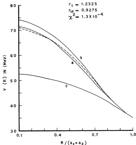
FIG. 3. Electrostatic potentials obtained from Eq. (2.3) (curve a) and Eq. (3.1) with  $R_c = a_t$  (curve b) and  $R_c = (a_t + a_p)$  (curve c) for the  ${}^7\text{Li}$ - ${}^{197}\text{Au}$  system. The results with minimum  $\chi^2$  given by Eq. (3.2) are shown as a dashed line.
