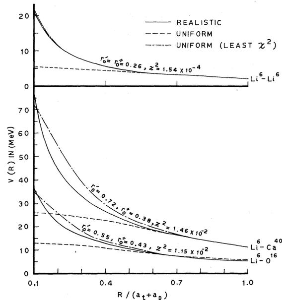
FIG. 5. Electrostatic potentials assuming realistic and uniform charge distributions for  ${}^6\text{Li}$ - ${}^6\text{Li}$ ,  ${}^6\text{Li}$ - ${}^{40}\text{Ca}$ , and  ${}^6\text{Li}$ - ${}^{16}\text{O}$  systems. The curves with minimum  $\chi^2$  defined in Eq. (3.2) are shown as dash-dotted lines.
