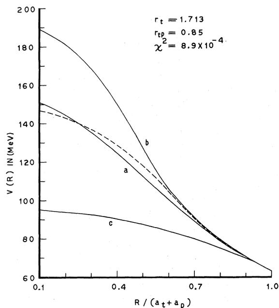
FIG. 2. Electrostatic potentials obtained from Eq. (2.3) (curve a) and Eq. (3.1) with  $R_c = a_t$  (curve b) and  $R_c = (a_t + a_p)$  (curve c) for the  $^{40}\text{Ca}-^{40}\text{Ca}$  system. The results with minimum  $\chi^2$  given by Eq. (3.2) are shown as a dashed line.
