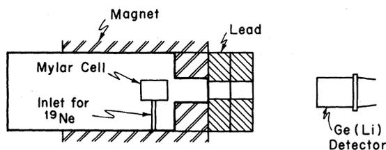
FIG. 1. Schematic of the  $^{19}\text{Ne}$  source and detector geometry. A second cell and detector (not shown) were used for normalization.
