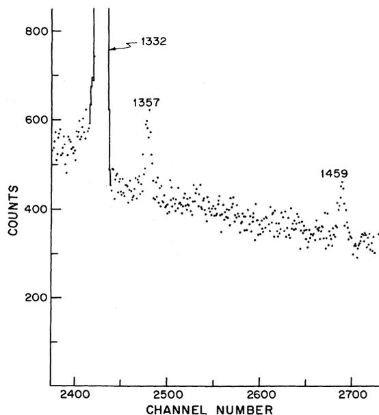
FIG. 2.  $\gamma$  ray spectrum from  $^{19}\text{Ne}$   $\beta$  decay. The peak at 1332 keV is from a  $^{60}\text{Co}$  calibration source and the peak at 1459 keV is from  $^{40}\text{K}$  contamination in the lead shielding.
