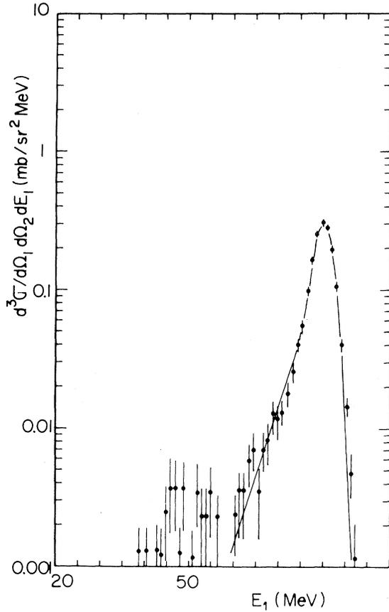
FIG. 2. The  $d^4\sigma$  spectrum for  ${}^3\text{He}(p, dp)p$  at  $\theta_a = 40^\circ$ ,  $\theta_p = -70^\circ$ , and  $E_2 = 68.5$  MeV. The experimental points are indicated with statistical error bars. The solid curve represents the PWIA calculation using the energy interval of 15 MeV and the  $d/\bar{d}$  ratio is  $3.50 \pm 0.5$ .
