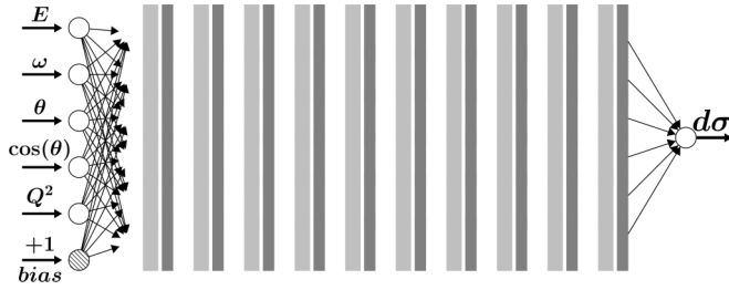
FIG. 2. The neural network architecture for model A. The light gray box corresponds to the hidden layer of fully connected neurons with ReLU activation function. The dark gray box denotes the batch normalization layer. In the output, there is the sigmoid function. In the architecture for model B, not depicted, each fully connected layer is followed by the dropout layer. In both models A and B, the network has ten layers of hidden units, consisting of 300 units each.
