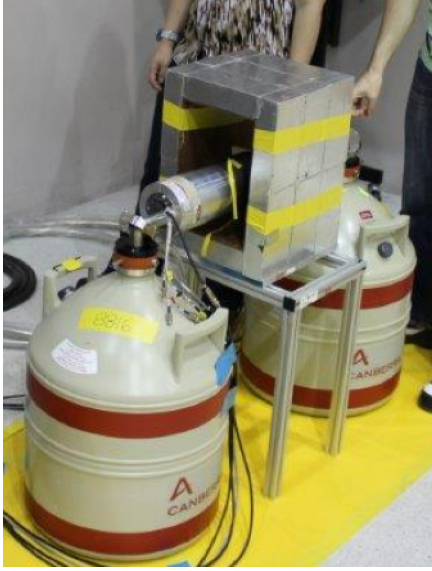
FIG. 3. Detector setup in the LLNL building near the Godiva-IV building. The HPGe detectors were oriented 180^\circ from each other facing the center of a copper-lined lead shield. This photo was taken during the July 2015 campaign.
