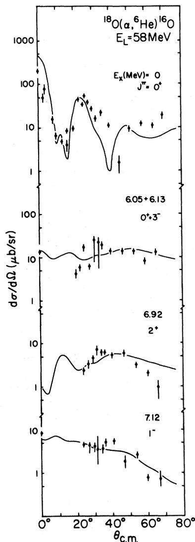
FIG. 2. Angular distributions for  $^{18}\text{O}(\alpha, ^6\text{He})^{16}\text{O}$ . The spin assignments are from other sources (see Ref. 5). The curves are DWBA calculations assuming a dineutron transfer (see text). The error bars include statistical errors and uncertainties in background corrections or peak unfolding.
