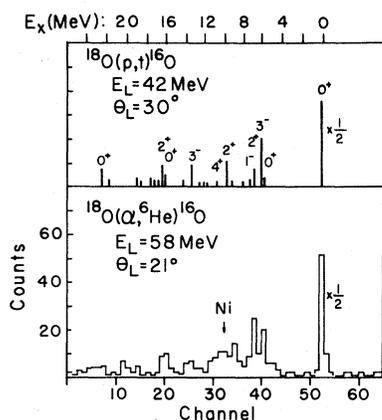
FIG. 1. Bottom: A  $^6\text{He}$  spectrum from  $^{18}\text{O}(\alpha, ^6\text{He})^{16}\text{O}$  taken with a nickel-oxide target and a  $\Delta E$ - $E$  counter telescope. The group labeled Ni is due to reactions from the nickel backing. Top: A schematic representation of an  $^{18}\text{O}(p, t)^{16}\text{O}$  spectrum (Ref. 5). Both the  $(\alpha, ^6\text{He})$  and  $(p, t)$  spectra were taken at  $L=0$  maxima ( $\theta > 0^\circ$ ).
